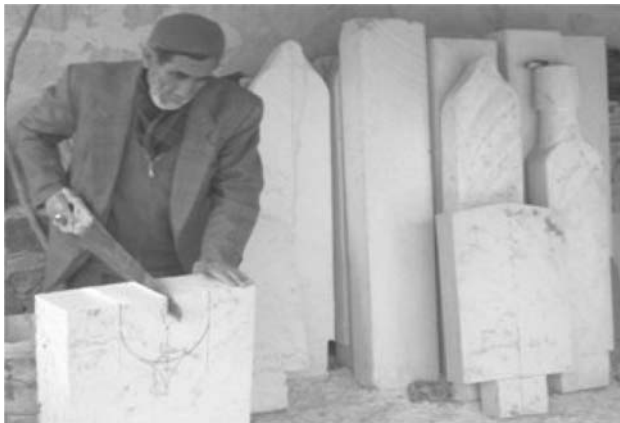
Fig. 4 A cut with handheld saw
