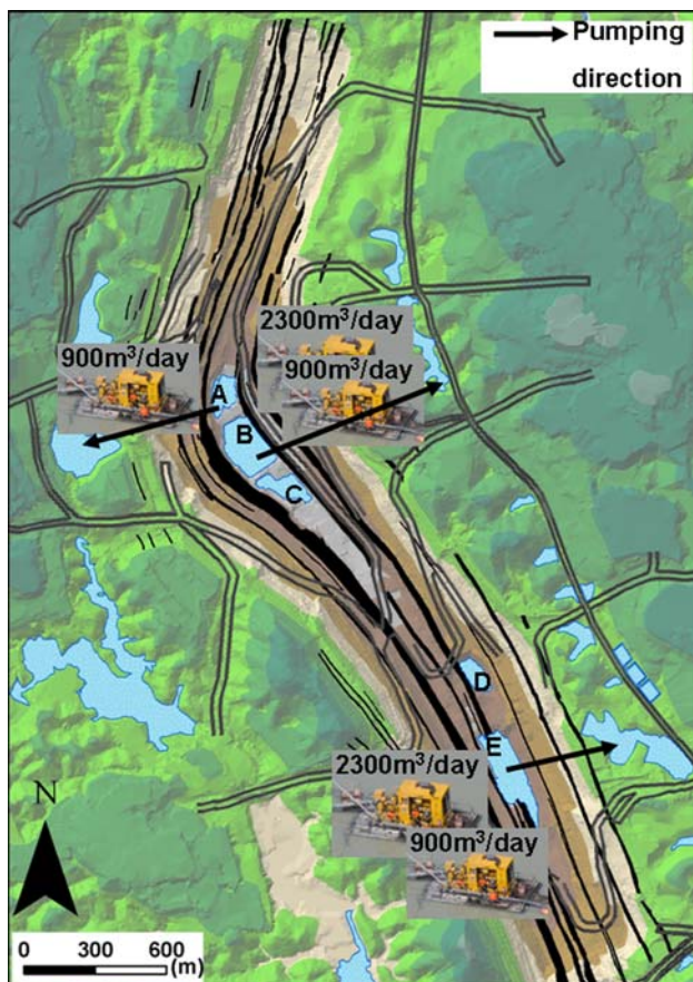
Fig. 6 Current allocation of pumping facilities on temporary storage ponds in the study area
