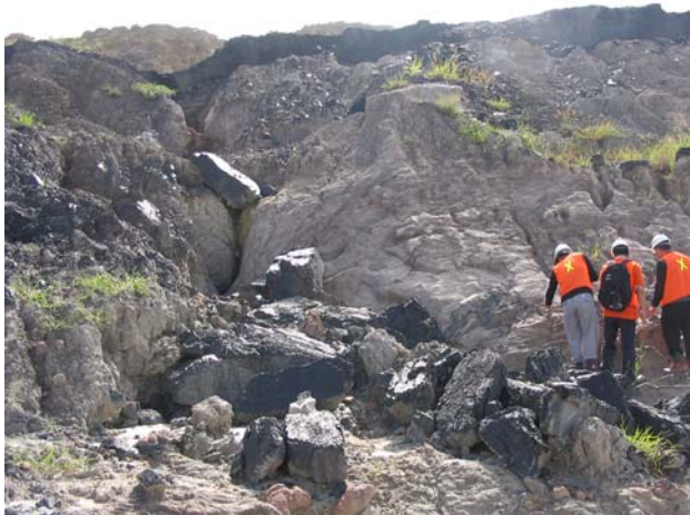
Fig. 11 Field survey in a vulnerable location derived from spatial analysis. The condition of the highly rated bench slope in Fig. 10c was highly unstable due to the valley created by concentrated surface drainage flows
