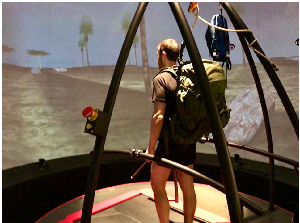
Fig. 1 The Computer Assisted Rehabilitation Environment (CAREN) is a fully immersive virtual reality system with a 6 degrees of freedom moveable platform, synchronized with virtual visual scenery projected over a 360° dome-shaped screen. A treadmill is embedded in the platform and its speed is synchronized with the visual flow. A surround sound system provides auditory stimuli congruent with the scenery. A motion capture system (Vicon) and set of force plates in the treadmill provide performance data. In the current study, participants walked while carrying a backpack weighing 30% of their body weight, and were safely secured to the system during the entire march. A bag of drinking water was available (hung on the upper right side of the metal frame)
