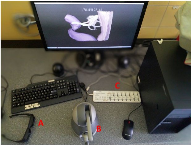
Fig. 1 VR temporal bone surgery simulator. a 3D glasses, b haptic device, c MIDI controller
