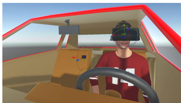
Fig. 3 The MR headset undergoes translations (indicated by the blue/green/red arrows indicating translations in x/y/z ) and rotations (indicated by the blue/green/red circles) relative to the interior of the vehicle. However, the vehicle also undergoes translations and rotations relative to the world, which may also be detected/conflated by the headset sensing (colour figure online)
