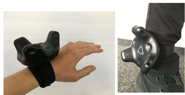
Fig. 5 For hand tracking, the Vive Tracker must be attached to the wrist (left). To track the leg movements, an additional Tracker must be strapped to the ankle (right)
