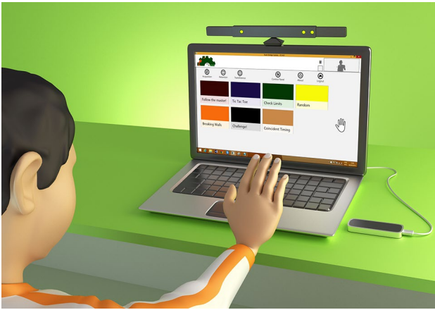
Fig. 1 Bridge Games main screen with seven games and options menu. The figure shows the use of Kinect or Leap Motion sensor for selecting an option. The selection can also be performed with the mouse, the tab key on the keyboard or the touch screen
