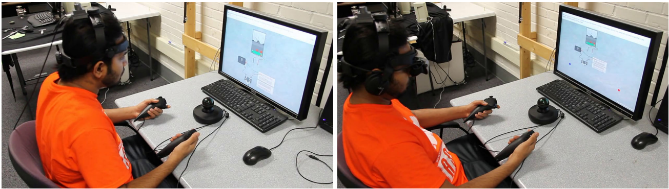
Fig. 1 Experiment setup for the Interactive Breadboard Activity Simulation in the DesktopVR condition (IBAS-DVR) on the left , and the IBAS-HMD condition on the right . The InterSense IS-1200 tracker is attached to the user’s head, and the user is holding a Razer Hydra controller
