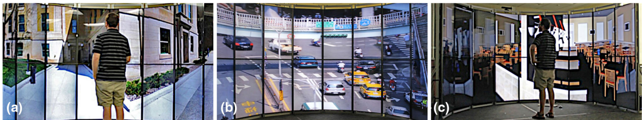
Fig. 3 The DSCVR System, shown displaying (a) high-resolution panoramic imagery, (b) playing 4K stereo video at 30 FPS using custom software, and (c) rendering an interior environment in real-time stereo 3D using the OGRE 3D engine
