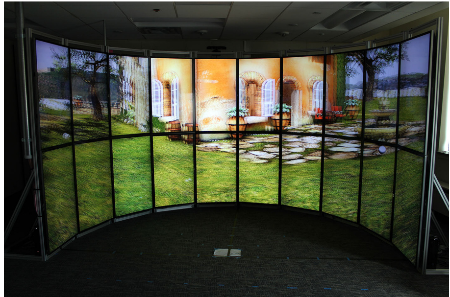
Fig. 3 The DSCVR System, shown displaying (a) high-resolution panoramic imagery, (b) playing 4K stereo video at 30 FPS using custom software, and (c) rendering an interior environment in real-time stereo 3D using the OGRE 3D engine
