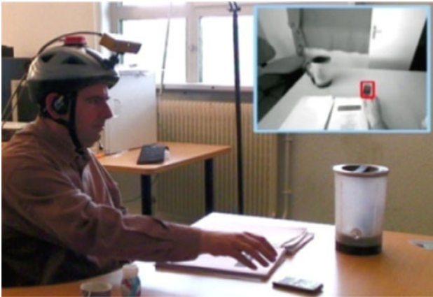
Fig. 7 The user interacts with the system via voice recognition; in this case, he would like to grab his phone, the system then activates the research of the corresponding models in the artificial vision module. If the object is detected, the position of the target is directly sent to the sonification module to display the position of the phone
