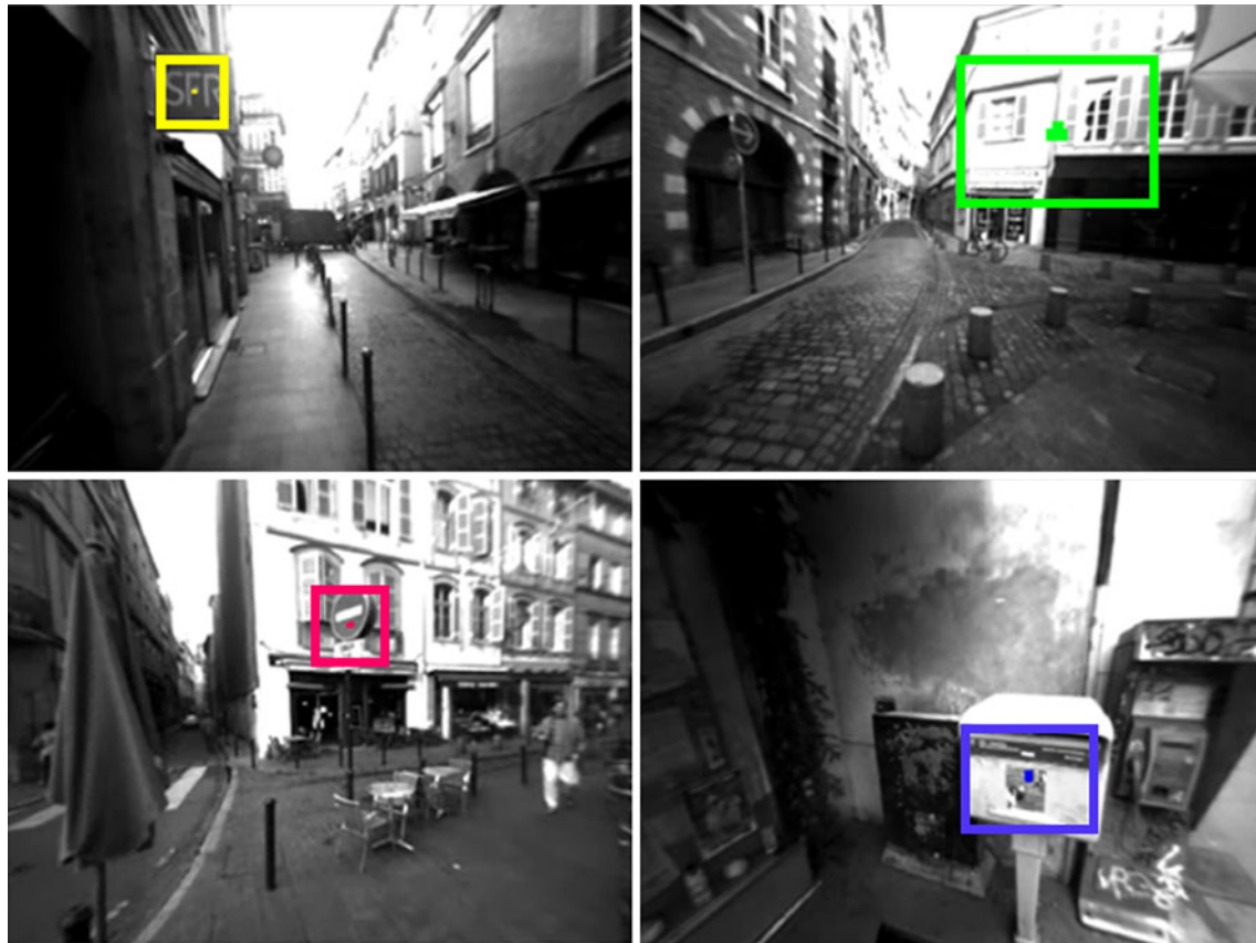
Fig. 3 Examples of geolocated visual landmarks used for user-positioning (shop sign, facade, road sign, mailbox)
