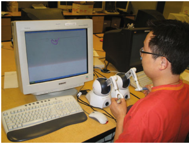
Fig. 16 The multi-modal experimental setup consisting of two haptic devices and graphical display
