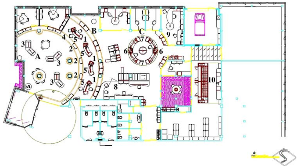
Fig. 8 The floor plan of the new pharmacy in case 2 by ProFarmaPlan architects (a waiting area, b counter area, and c prescription area)
