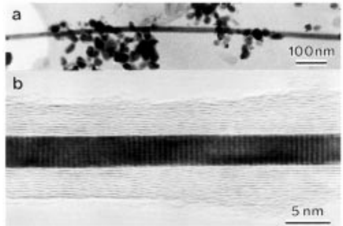
Fig. 11. (a) TEM image of a long typical filled carbon nanotube obtained with a high purity carbon anode doped with Cr and S in a S/Cr = 0.5% atomic ratio. (b) HRTEM image of another Cr-containing nanowire having a very small diameter and encapsulated in 10 graphitic layers. The filling is single-crystalline and in epitaxial relationship with the graphitic walls.
