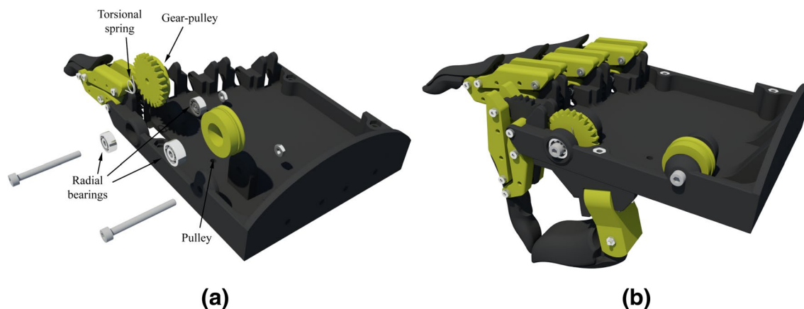
Fig. 4 Design of the movement transmission system detailing internal parts and fully assembled hand design
