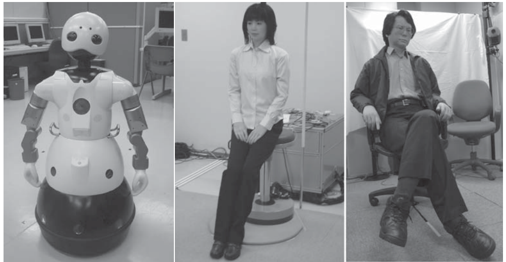
Fig. 1. Three categories of humanlike robots: humanoid robot Eveliee P1 ( left : developed by Osaka University), android Repliee Q2 ( middle : developed by Osaka University and Kokoro Corporation), and Geminoid HI-1 ( right : developed by ATR Intelligent Robotics and Communication Laboratories)
