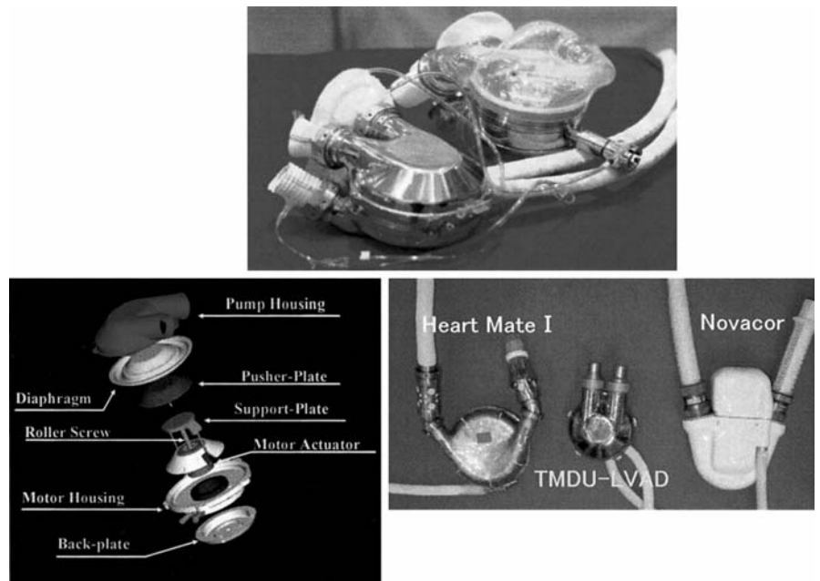
Fig. 22. Electromechanical replacement type MCSD in comparison to AbioCor (top) and single ventricle MCSD of Tokyo Medical and Dental University in comparison to Novacor and HeartMate I VE
