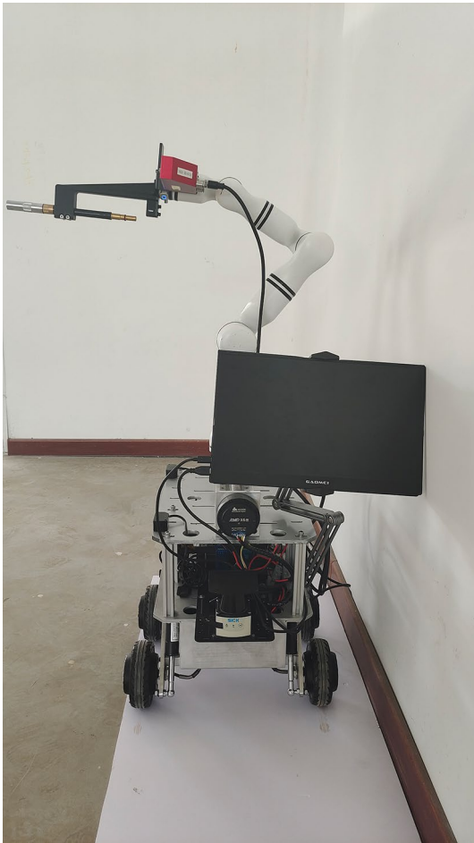
Fig. 10 Schematic diagram of welding robot
