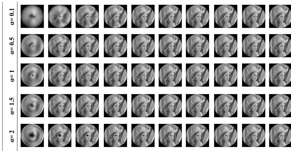
Fig. 12 Recursive computation of AFPJFMs’ reconstructed grayscale image Lena ( 128 \times 128 ) with order K = 5, 10, \dots, 50 from left to right and \alpha = 0.1, 0.5, 1, 1.5, 2 from top to bottom
