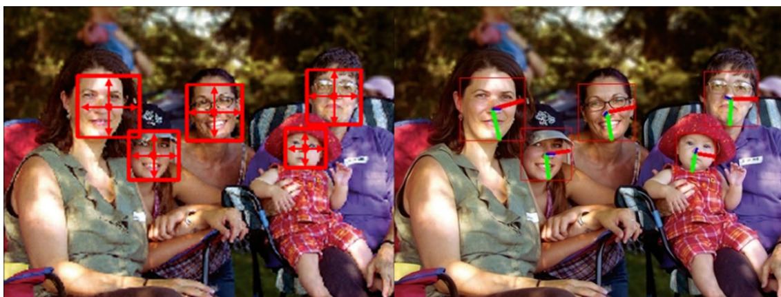
Fig. 1 We detect the face as a point and calculate the size of the face bounding box and the head pose of the face directly at this point
