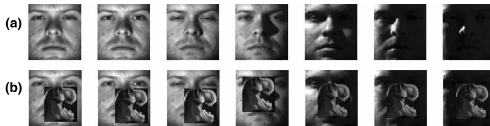
Fig. 11 Partial face images of the same subject taken from the Extended Yale B database. a Shows the non-occluded images of one subject, and the corresponding images were artificially occluded by a dinosaur patch at random position in (b)
