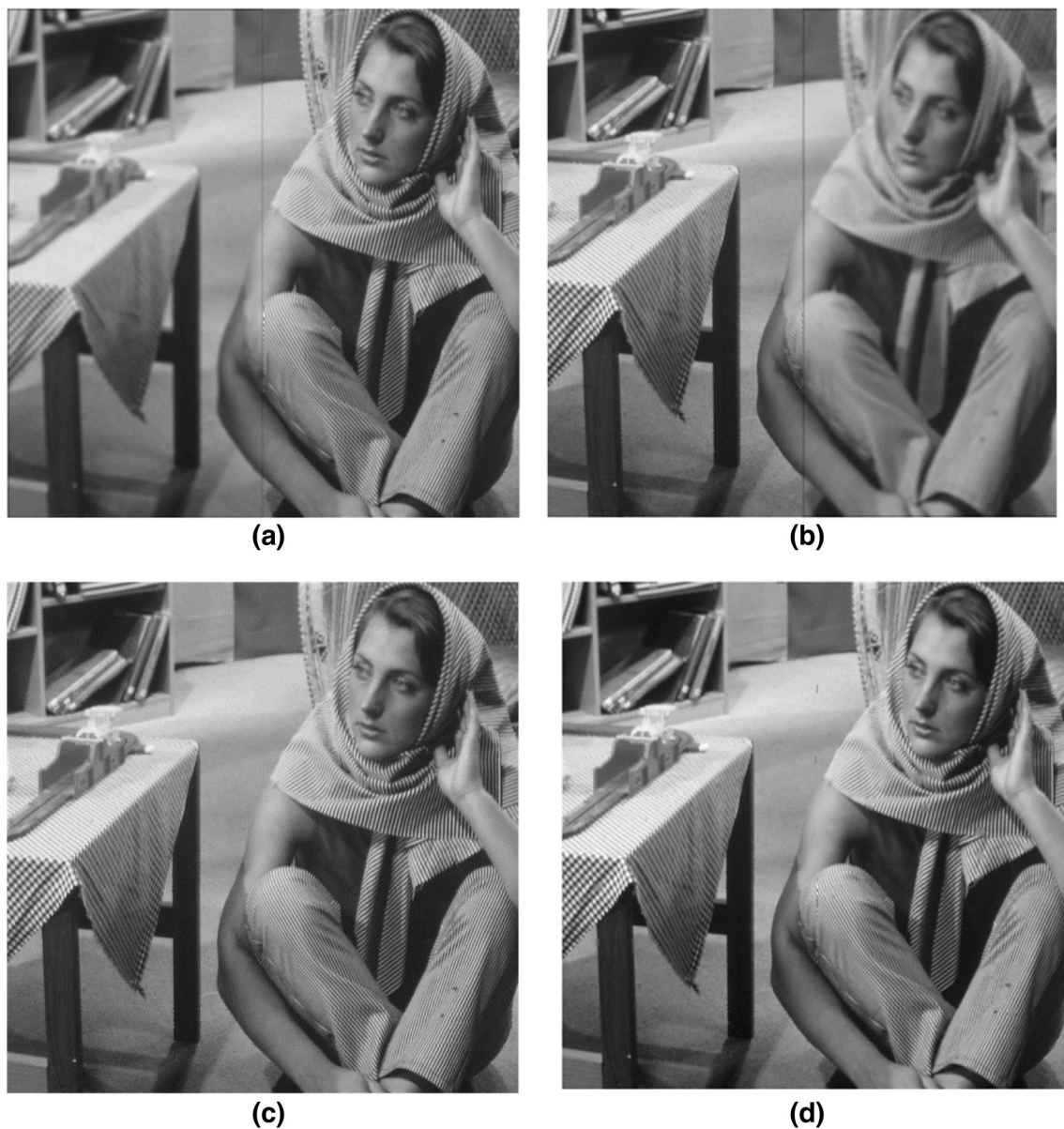
Fig. 6 a Right focussed, b left focussed, c original image, d fused using RF
