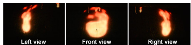
Fig. 12 Aerial image using a piano wire for hanging the acrylic plate, viewed a from the right, b in front, and c from the left
