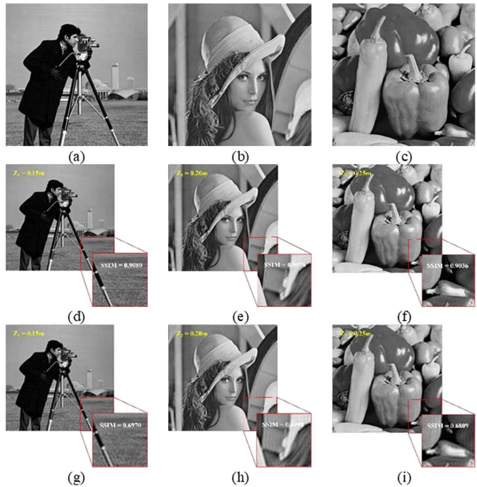
Fig. 4 a–c Original images, reconstruction results of d–f using a 400 × 400 pixels cross-shaped filter, reconstruction results of g–i using an 800 × 800 pixels rectangular filter
