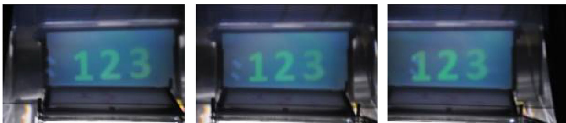
Fig. 13 Aerial three-layered display. The screen showing 123 is floating over the half mirror
