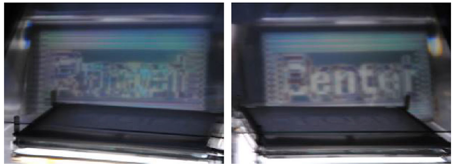
Fig. 14 Aerial display results of the front , the middle , and the rear images, when the other two LCD panels were black
