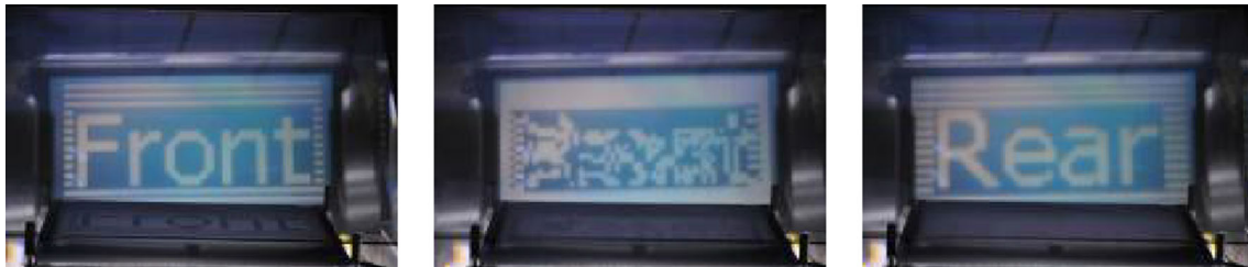
Fig. 14 Aerial display results of the front , the middle , and the rear images, when the other two LCD panels were black
