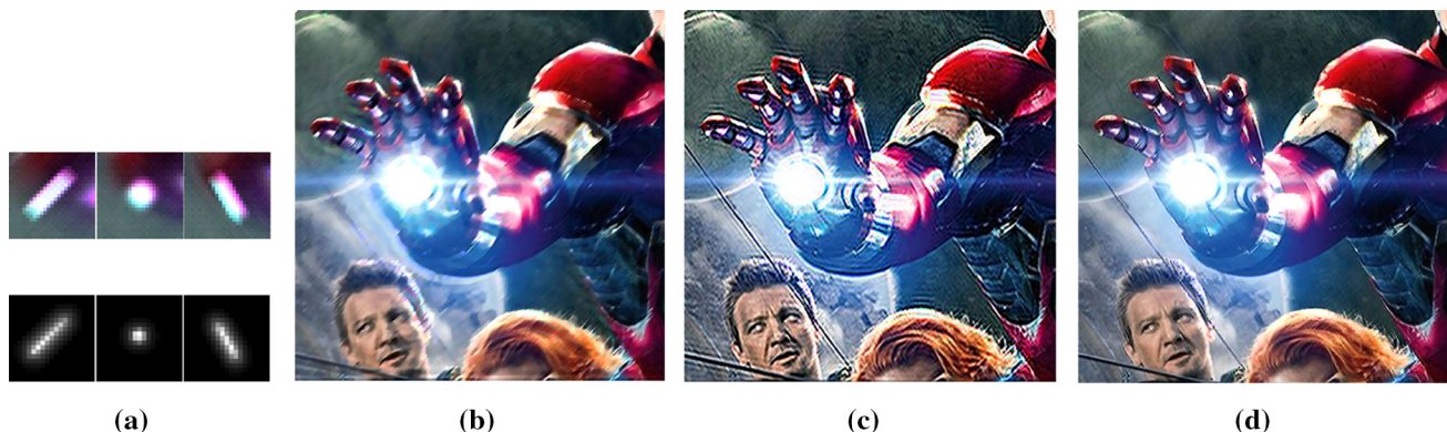
Fig. 5 a The top three are the light streaks we detected, the bottom three are the PSFs estimated, b–d the restored image using Refs. [19, 22] and ours respectively
