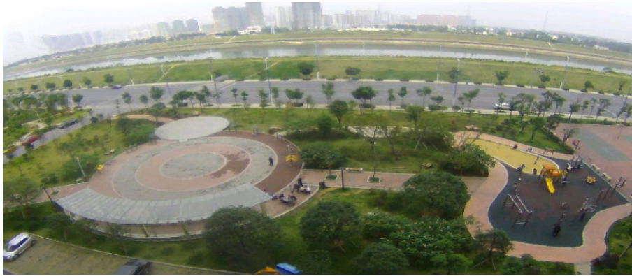
Fig. 3. (Color online) The fish-eye panoramic image captured by master–slave visual surveillance system, which has obvious distortion in horizontal direction.
