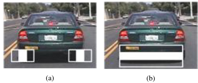
Fig. 2. (Color online) Haar-like features of front vehicles: (a) rear-wheels, and (b) shadow under vehicles.
