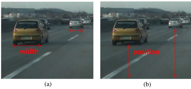
Fig. 7. (Color online) Two distance estimation methods: (a) the width-based method and (b) the position based-method.
