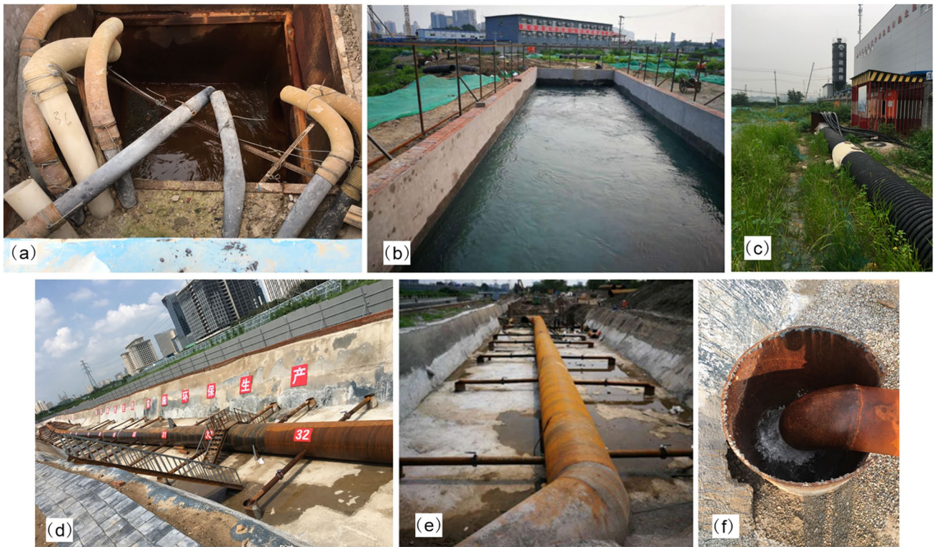
Fig. 5 Test equipment for the multi-well pumping-recharge tests: a abstraction collection tank; b sedimentation tank; c transportation pipe; d recharge site; e recharge collection pipe; f recharge well
