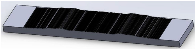
Fig. 3 3D printing template with typical rough profile (JRC = 8–10)
