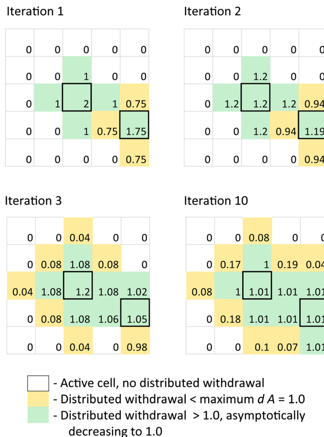
Fig. 1 Distributed withdrawals for iterations 1, 2, 3, and 10 on an example footprint grid. The product of the depth-rate index and the cell area, dA = 1 . The input (iteration 0, not shown) withdrawals are zero in all cells except for the outlined cell (3rd column from left, 3rd row from top)
