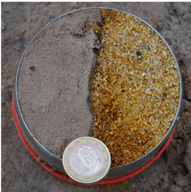
Fig. 4 Sample cylinder (diameter 8 cm) recovered from the annulus of a dewatering well in the open-pit lignite mine Garzweiler, Rhineland, Germany, (plan view) with (from left to right): aquifer (grey), filter cake (dark), gravel pack with iron incrustations. Photo: RWE Power AG, with permission
