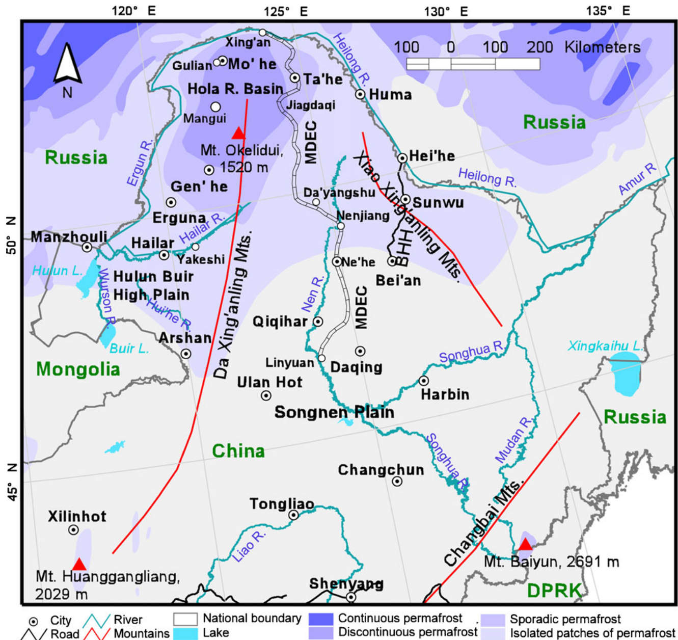
Fig. 4 Map of permafrost in northeast China. Note 1: MDEC is the Mo'he-Daqing Engineering Corridor, which includes highways, railways, crude oil pipeline, power transmission lines, and other linear infrastructures. BHH is the Bei'an-Hei'he Highway. DPRK is the Democratic People's Republic of Korea (North Korea). Songnen Plain is the major plain in northern part of northeast China, which was formed by the alluvial and fluvial plains of the Songhua and Nen rivers, major tributaries of the Heilong-Amur River. The Hulun Buir High Plain is named after the sister lakes of Hulun and Buir lakes, which were formed by the tributaries of Hailar River. Note 2: Traditionally, permafrost in northeast China is regarded as latitudinal permafrost because of higher northern latitudes in northeast China. However, permafrost is mainly distributed in the northern Da Xing'anling Mountains, with Mt. Okelidui (1,520 m a.s.l.) as the highest peak, and Xiao Xing'anling Mountains. These mountains are generally low, with elevations of several hundreds of meters. In the southernmost Da Xing'anling Mountains, with the highest peak at Mt. Huanggangliang (2,029 m a.s.l.), and in the Changbai Mountains, with the highest peak at Mt. Baiyun (2,691 m a.s.l.), permafrost is generally classified as elevational. However, a unanimous understanding is not yet reached among Chinese geocryologists
