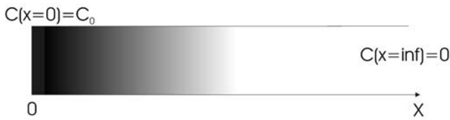
Fig. 2 Boundary conditions for the analytical solution
