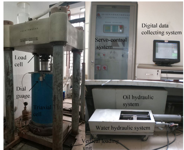
Fig. 2 The large-scale triaxial testing apparatus
