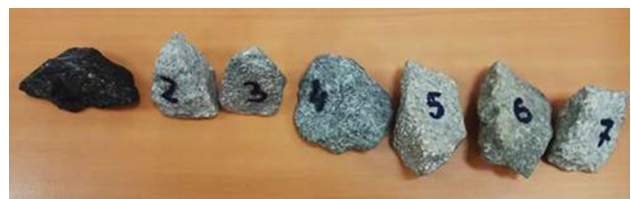
Fig. 1 Sample of seven ballast grains used for the morphology analysis. For identification purposes, grains were named as SX, being X the number noted on the grain surface
