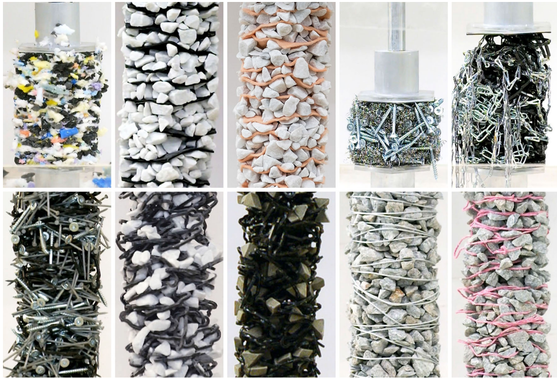
Fig. 7 Experiments with a wide range of different jammed material systems. Gramazio Kohler Research, ETH Zürich, 2014
