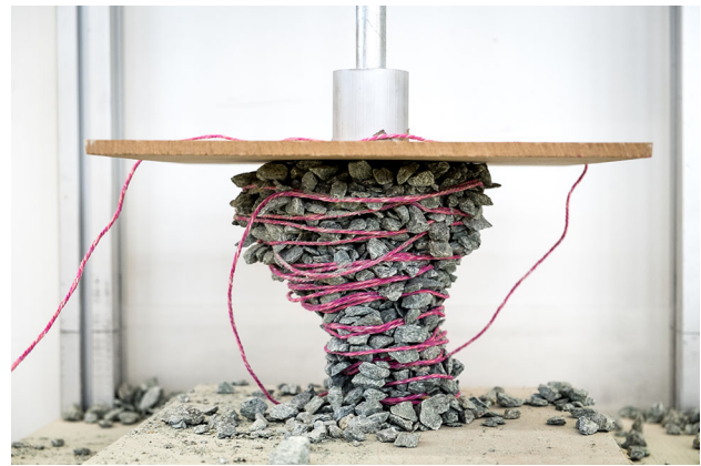
Fig. 8 Rock print, demonstrating how the jammed aggregates can be shaped into geometrically and structurally sound designs. Gramazio Kohler Research, ETH Zürich, 2014
