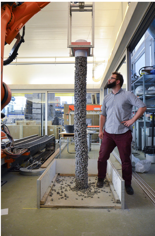
Fig. 16 Picture showing a jammed column (2100 with 180 mm diameter) produced with a six axis KUKA KR 150 L110 robot mounted on a linear axis, and equipped with a custom mould end-effector. Gramazio Kohler Research, ETH Zürich, 2015
