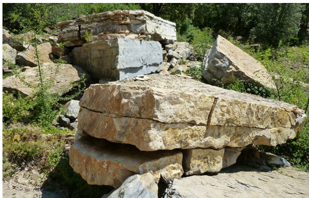
Fig. 2 Examples of somewhat rectangular blocks observed in a rock-fall near Millau, France (from Cuervo et al. [4])
