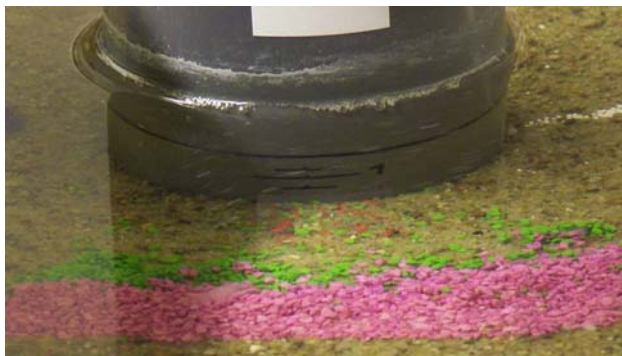
Fig. 6 Red markers appearing back into the soil surface
