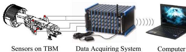
Figure 16 Condition monitoring system
