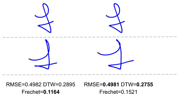
Fig. 11 Metrics comparison. On the top, the ground truth and on the bottom two predictions coming from different models
