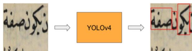
Fig. 4 YOLO inputs a patch of size 320 \times 320 and predicts the bounding boxes of subwords within the patch
