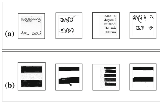
Fig. 5 Sample images from Real Document Image Dataset: a Input images; b corresponding ground truth images
