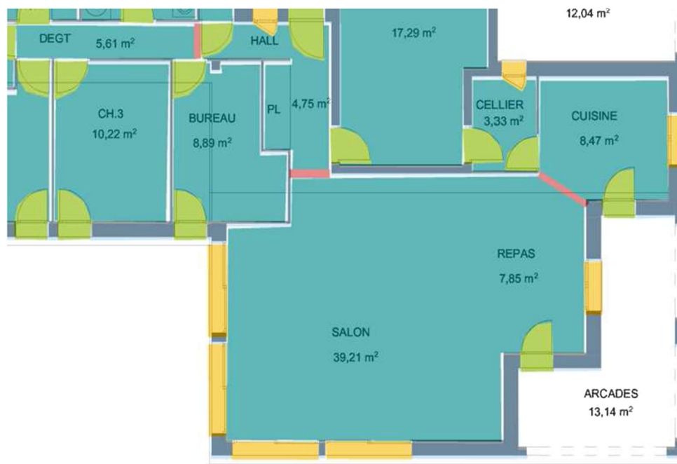
Fig. 6 Rooms labeling. Rooms are drawn in turquoise and separations in red (color figure online)
