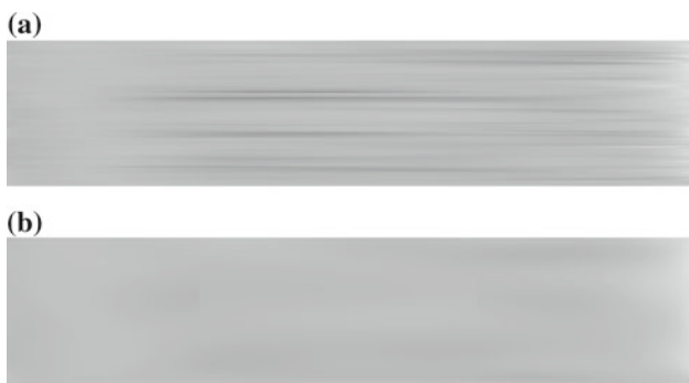
Fig. 3 Document background surface estimation: a The document background surface that is estimated through the row-by-row polynomial smoothing procedure; b The final document background surface that is estimated after the column-by-column smoothing procedure
