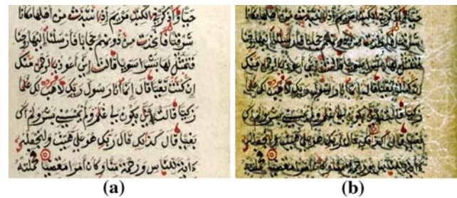
Fig. 2 Sample input scanned and back-lit images—part of a page. The back-lit image shows verso inscription and details within the paper—watermark features are in the right hand margin
