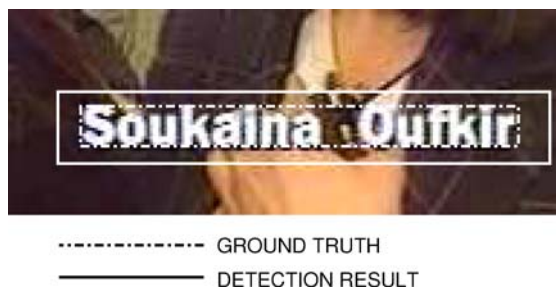
Fig. 3 An example rectangle detected with area recall = 100% and area precision = 50%
