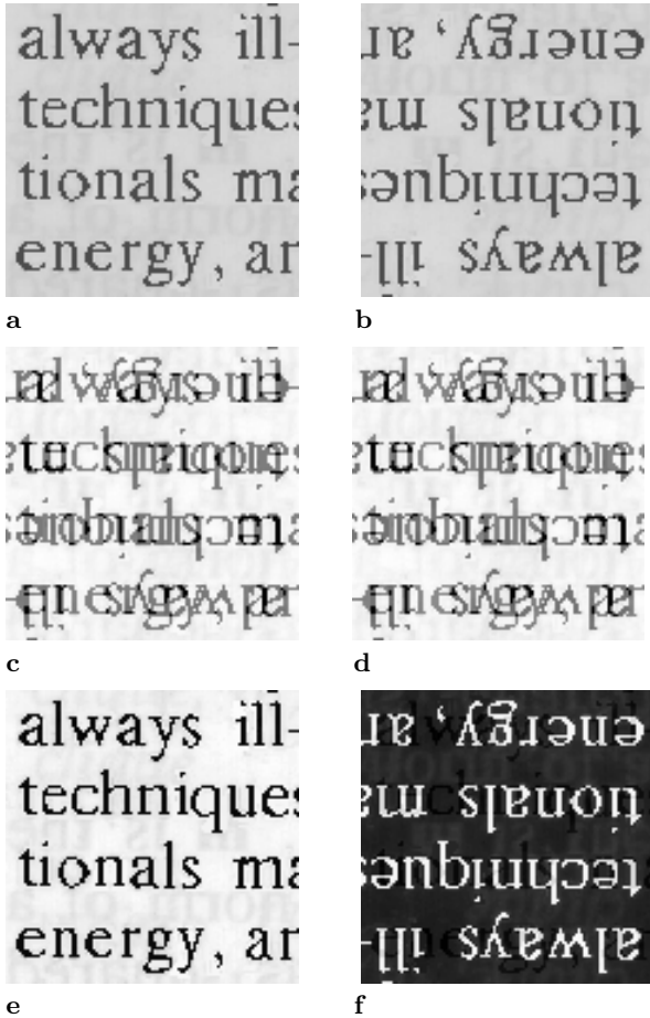
Fig. 1. Synthetic noiseless example. a First original image. b Second original image. c First mixture. d Second mixture. e First FastICA output. f Second FastICA output
