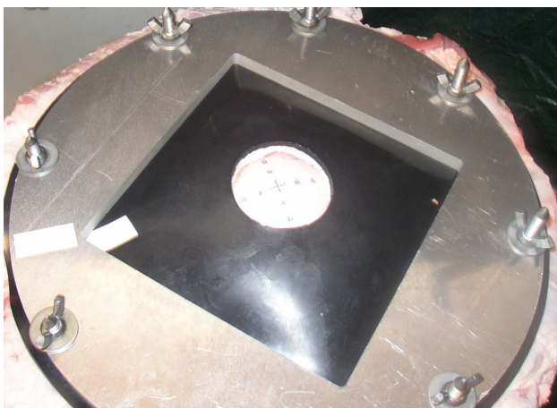
Fig. 1 Device mounted with the EPDM membrane in situ being fixed to the pig belly by screws and bolts reliably. The white mark on the left indicates the direction of the linea alba. The dots on the mesh are used to observe the direction and length of migration in relation to the linea alba before dislocation may occur
