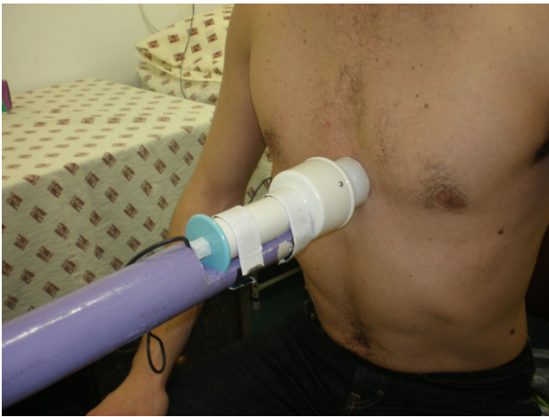
Fig. 1 Set-up of the wall-mounted dynamometer for ITFS measurements
