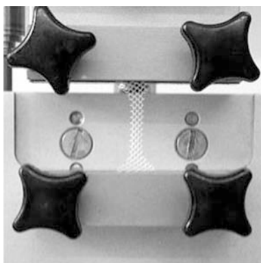
Fig. 2 Tensile-test specimen. View of the two gripping jaws with clamped surgical mesh punched in hourglass form
