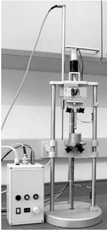
Fig. 4 Tensile-test device with applied punching test adapter (clamping ring and spherical punch)
